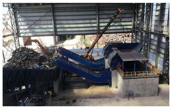
The BRAVO 'redripper', with horizontally counter-rotating shafts, is used upstream of hammer mills in scrap mills, to coarsely and homogeneously crush mixed scrap, bulky scrap and E.L.V. It is in particular used to rip bales of E.L.V., light and collected scrap, to facilitate feeding and make uniform the subsequent ripping operation at the mill.
